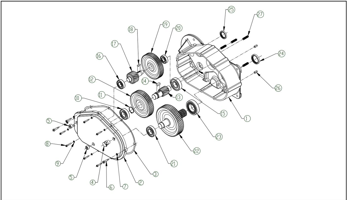
Figure 9-2. Hoist Gearing
