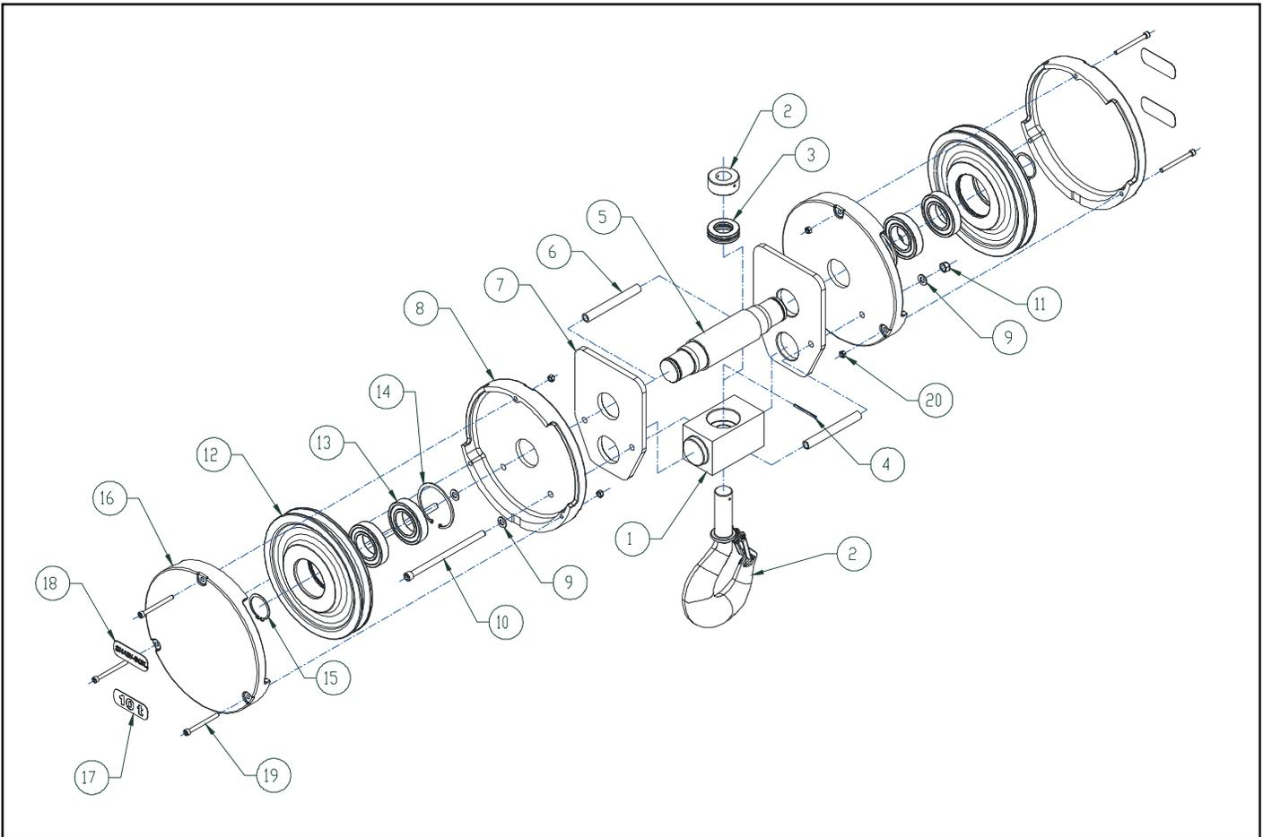
**Figure 9-4a. Lower Block Assembly
