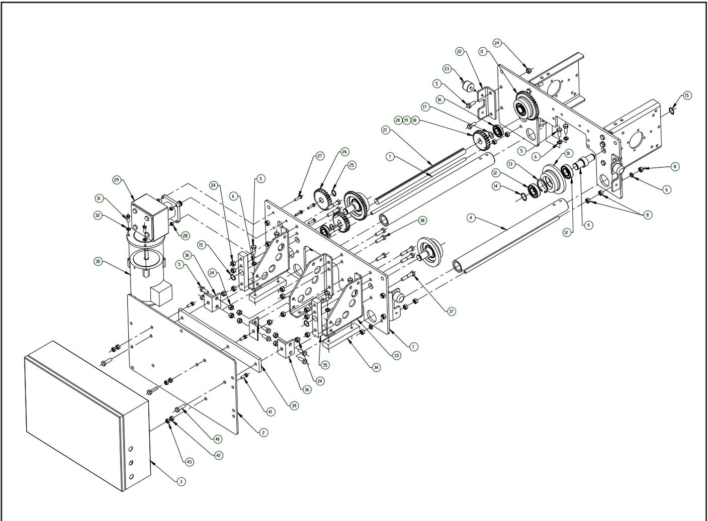
Figure 9-3. Motor Driven Trolley Frame and Drive
