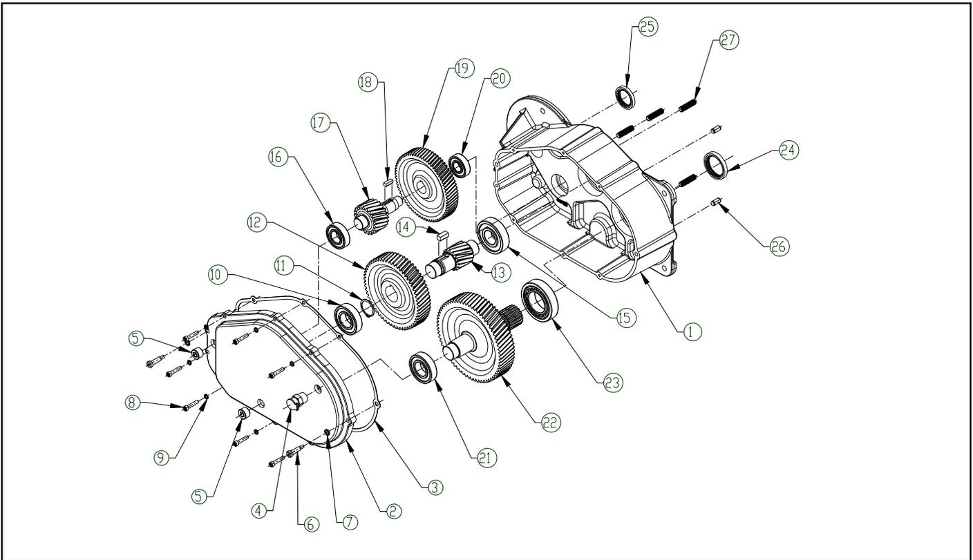
Figure 9-2. Hoist Gearing
